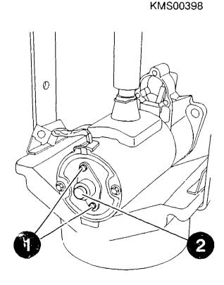
Disassembling commutator end shield
